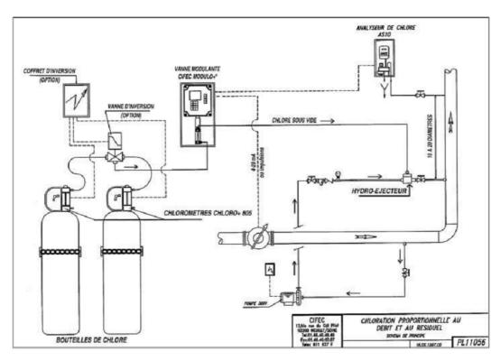
The 4-20 mA signal given by the internal controller is compared to the valve's position. It follows an automatic opening or closing by an endless step to step motor until concordance between the position and the electric order signal.
